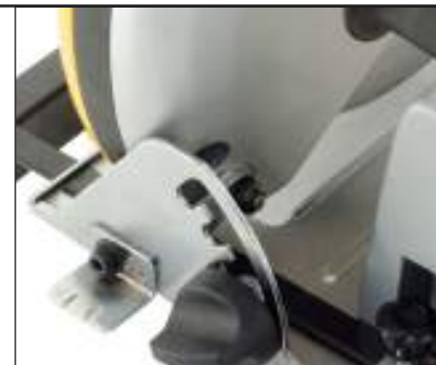
Mitre cuts up to 45° (type 5 1115 and 5 1116)
