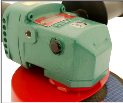
Lock button for changing the grinding discs
