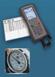
pressure and automatically re-adjusts the pressure when the auto repump mode is enabled. For example as a bolting joint settles the pressure will drop and therefore the pressure will be replenished.
